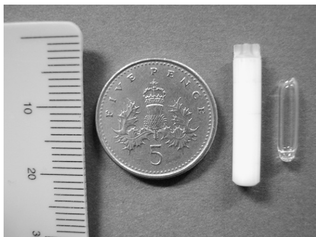
Fig. 1. Photographic size comparison of a glass insert, a standard 4 mm rotor and a 5p coin.
